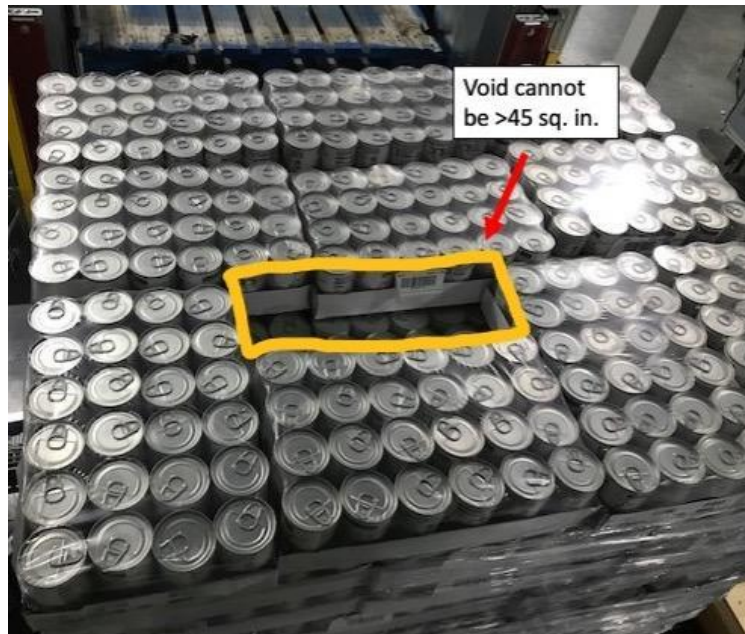
Figure 11: Unacceptable Void Space
