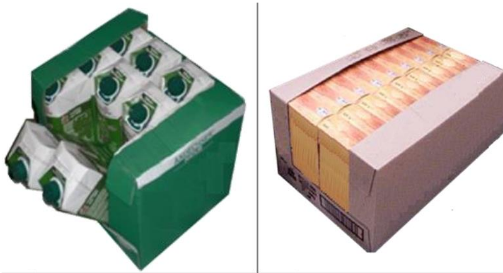
Figure 7: Poor versus optimal open top packaging
